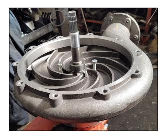
Insert 2 bolts of sufficient length into the holes in the impeller to be able to push on the bottom of the pump casing and thus extract the impeller from the shaft.
