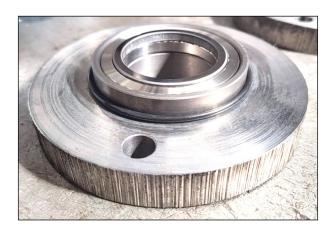
For reassembly, insert the new seal into the seal holder.
