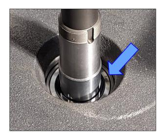
Similarly, check the condition of the fixed seal at the bottom of the pump body.
