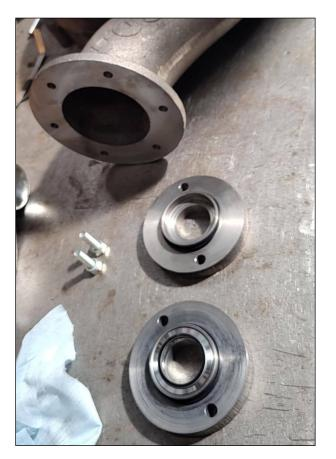
Inspect the condition of the stationary seal, checking as for the rotary seal for scratches, signs of overheating and streaks, remove the seal and check the condition of the round rubber gasket and the seal cover gasket.
