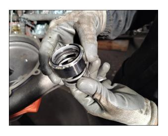
Now take the new rotary seal and slide it onto the pump shaft until it makes contact with the fixed seal.
