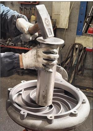
We now insert the impeller onto the conical shaft.
