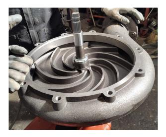
Tighten the impeller locking ring with a suitable spanner.
