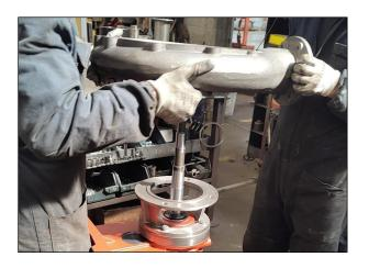
Remove the pump body from the shaft and place it on the bench on the access side of the fixed seal.
