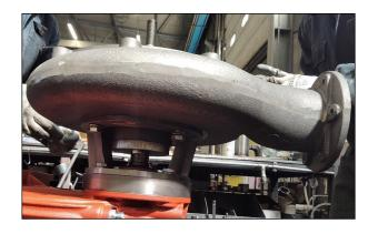
To continue with seal replacement, unscrew the 4 bolts securing the pump body to the gear box mount.
