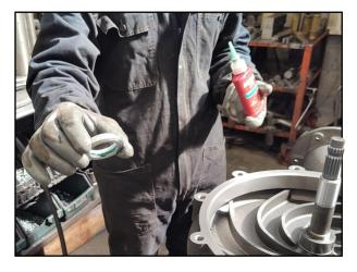
Screw in the ring nut, taking care to spread threadlock (loctite or similar) on it.
