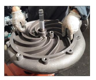
When you notice that the impeller has come out of the seat on the conical shaft, pull it out of the pump body.
