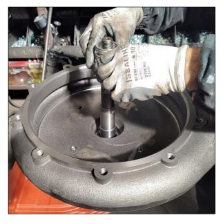
Pull the rotary seal off the shaft.
