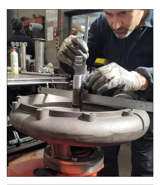
Once the pump casing is fixed, take a depth gauge and measure the distance
