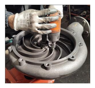
Alternately tighten the two bolts so that the impeller is gradually pulled out.
