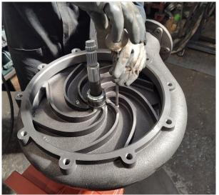
Close the extraction holes of the impeller with the grub screws.
