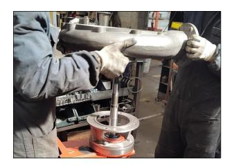
Refit the pump housing to the unit and secure it with the four bolts.
