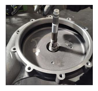
At this point, the rotating seal is visible: remove the impeller locking key from the shaft.
