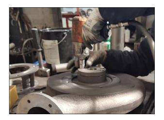
Unscrew the two bolts securing the fixed seal holder.
